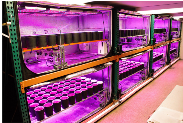
Fig. 6. Deployment of robotic gantries for carrying out large factorial experiments. In this setting, machines are stacked in commercial shelves, and enclosed into tents that allows for the control of temperature and CO 2 concentration.
